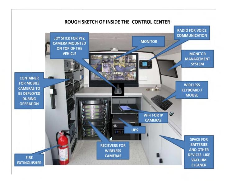
ABOVE: PICTURE of MOBILE SURVAILLANCE VEHICLE'S INSIDE LAYOUT
